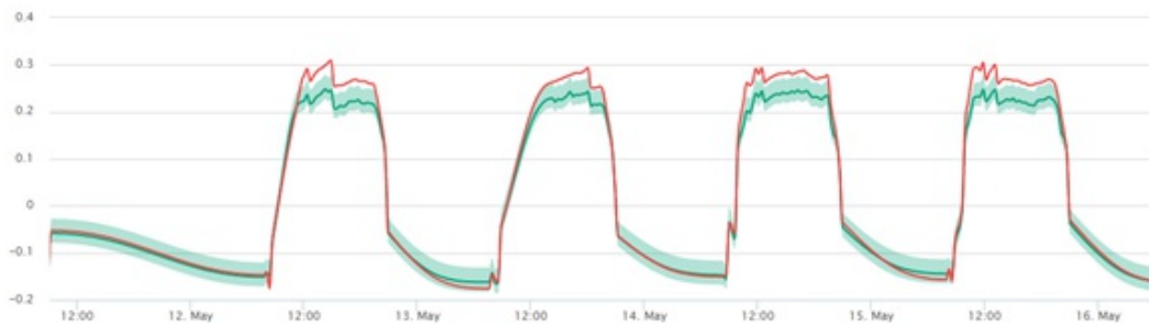
Figure. The displacement of the central axle of a compressor is measured (red) and modeled (green) with the confidence interval of the model (light green). It is seen that the model accurately models the behavior of the machine even during load changes, both to increased and decreased load. We observe a deviation between model and measurement at full load each time that full load is reached. This is an indication of a machine problem and will be alarmed.
